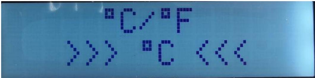
This interface is the temperature setting interface. Turn the knob to change the system temperature unit °C/°F; press the knob to confirm the change and enter the next setting.
