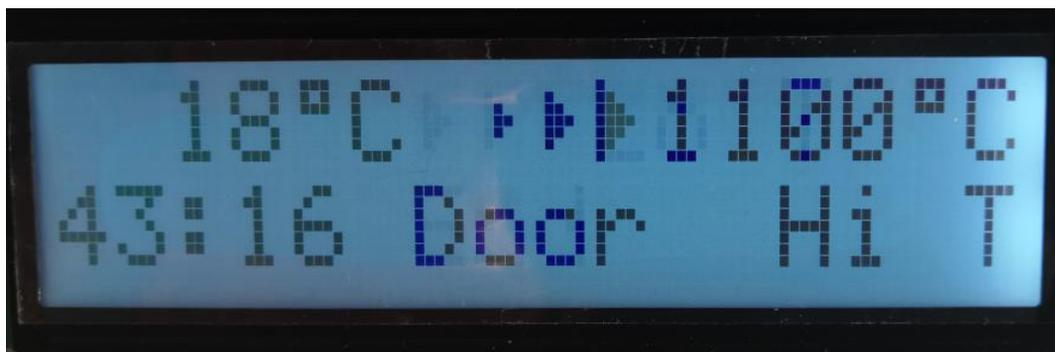
The electric furnace will beep and timed. If the furnace door is closed within 5s, the sintering process will continue; if the furnace door is not closed within 5s, the sintering process will automatically end.
